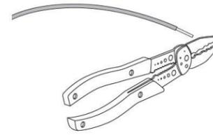
When replacing existing devices, label wires before disconnecting. Disconnect old device.
